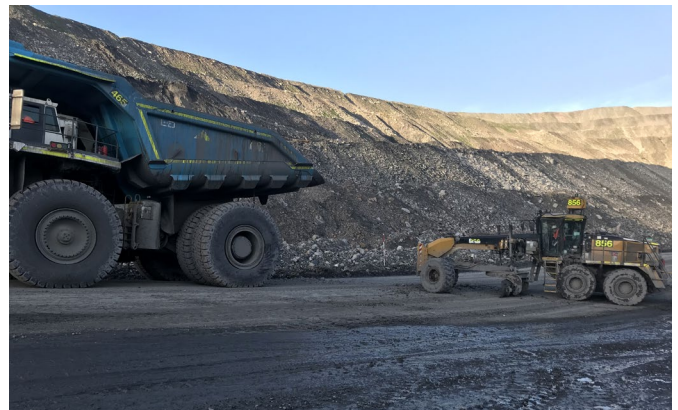
Figure 2 Contact between haul truck and grader
