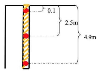
Figure 4. Loading pattern of a 5.5m deep monitoring hole.
