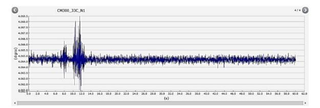
Figure 7 : Example of the dynamic evolution of a crack with no effect
