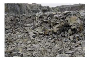
Figure 15. Blast 110b5011: coarse fragmentation at the blow out location.
