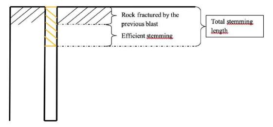
Figure 19. Definition of efficient and optimal stemming lengths.
