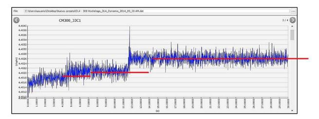
Figure 12 : Example of the vibration of a crack with multiple opening evolutions
