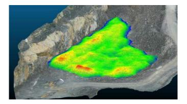
Figure 2. Swelling field displayed on the 3D model created before blasting. (Blast N°110b3003)
