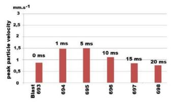
Figure 8. Grafical presentation of measured maximum values of peak particle velocity x at the standpoint S12 (buiding object No. 91 in the village Trebejov) at millisecond timing.
