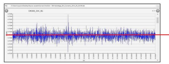
Figure 9 : Vibration of a crack with no evolution
