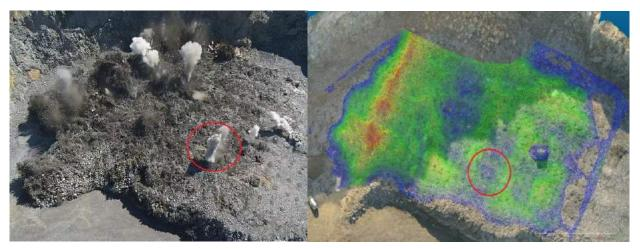
Figure 14. Blast 110b5011: correlation between stemming blow outs and smaller swelling.
