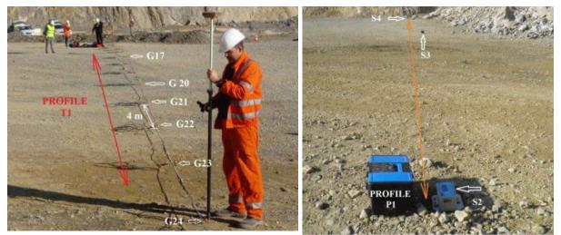
Figure 3. Measurement of seismic profile position T1 at the III. Etage with the seismic apparatus Terraloc Mk 8 during the measurement of propagation velocity of seismic waves at No. 693 and 694 in the quarry Trebejov. Position of the vibrograph Vibraloc ABEM at the measuring profile P1, standpoint S2 at the distance 26,5 m from the borehole mouth V1 measuring the vibration velocity during the experimental blasts No. 693 and 694 in the quarry Trebejov.
