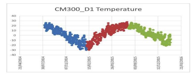
Figure 6 : Evolution of the temperature near a crack
