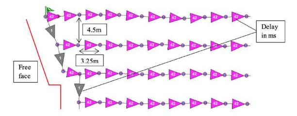
Figure 9. Sequence used in a standard blast (Nonel sequence).
