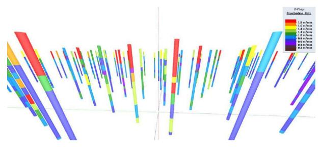
Figure 6. Display of penetration rate for each hole in Expertir.
