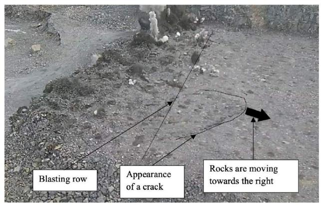
Figure 16. Blast 110b5012: effect on a crack in the rock mass seen on the video.
