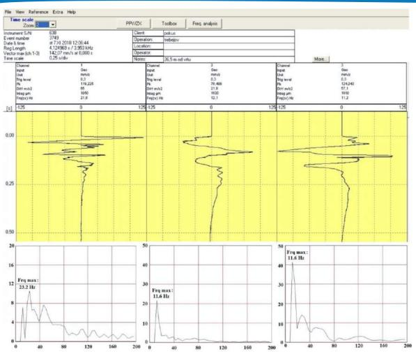
Figure 6. Grafical record and frequency analysis of particular vibration components according to the measurements at the standpoint S2 (26,5 m from the blast) in the quarry Trebejov – seismic apparatus ABEM Vibraloc at the experimental blast No. 693 at the profile P1. The first channel-z, the second channel-x, the third channel-y at the standpoint No. 693.
