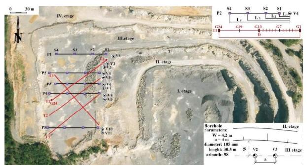
Figure 2. Position of experimental blasts No. 693 (V1), No. 694 (V2,V3), No. 695 (V4,V5), No. 696 (V6,V7), No. 697 (V8,V9) and No. 698 (V10, V11) in the quarry Trebejov in relation to the measuring profiles P and T.  $L_1$ =32,5 m  $L_2$ =40 m,  $L_3$ =60 m,  $L_4$ =80 m. Distance between G1 and G13 = 48 m, between G1 a G24 =96 m.
