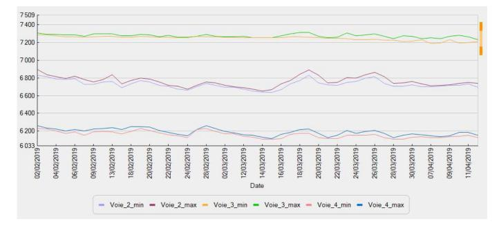
Figure 4a: Example of the evolution of the opening of a crack
