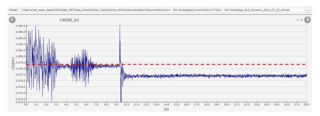
Figure 13: Example of the vibration of a crack with a closing evolution
