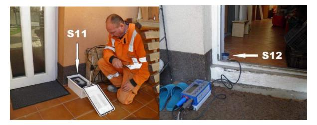
Figure 4. The monitored building object No. 91 in the village Trebejov and the measuring standpoint S11 and S12 at the entrance to the building object No. 91, wih the position of three-component vibrograph Mini-SuperGraph and Minimate Pro 6 in the village Trebejov.
