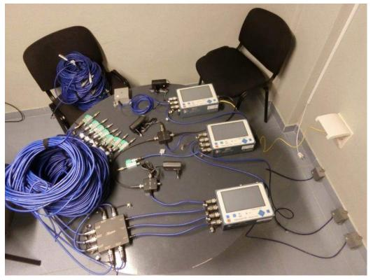
Figure 1 : Example of a system with geophones and accelerometers
