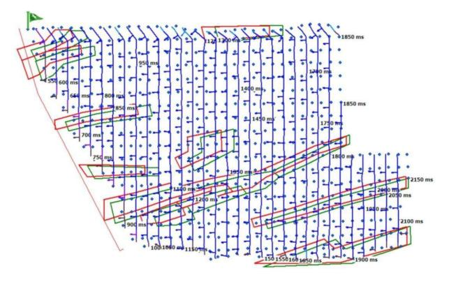
Figure 10. Correlation between ore movement (green: initial position, red: final position) and isochrones (in blue).
