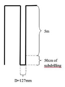
Figure 8. Drill pattern used for a standard blast.
