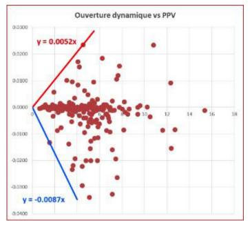
Figure 15 : Example of the dynamic opening correlation (Y axis)/PPV (X axis)
