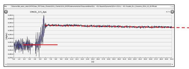
Figure 10 : Vibration example of a crack with a simple evolution
