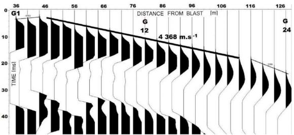
Figure 7. Seismic record accomplished with measuring apparatus Terraloc Mk8 of the profile T1 at the measuring standpoint No. 693 with identified propagation velocity of seismic wave 4368 m.s-1, frequency 24 Hz in the rock medium of the dolomites in the quarry Trebejov
