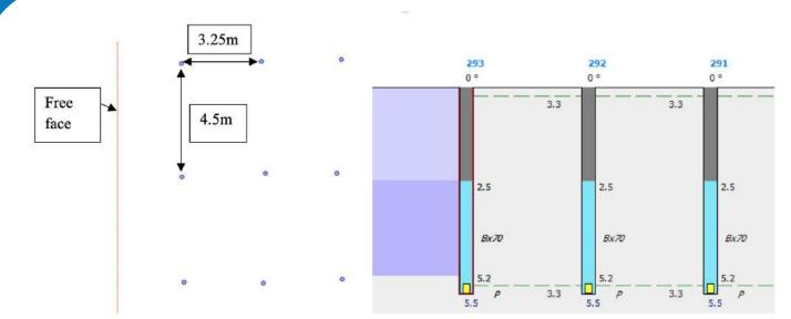
Figure 7. Hole pattern and loading plan for a standard blast.
