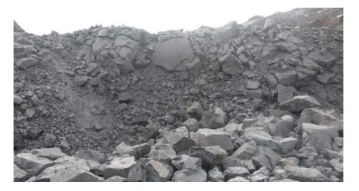
Figure 11. Coarse fragmentation at the top of the muckpile from blast 115g3011 with 2.7 m stemming.
