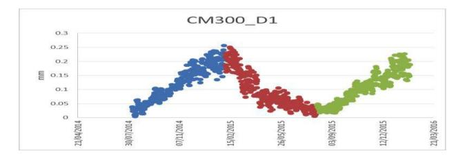
Figure 5b: Example of the evolution of the opening of a crack
